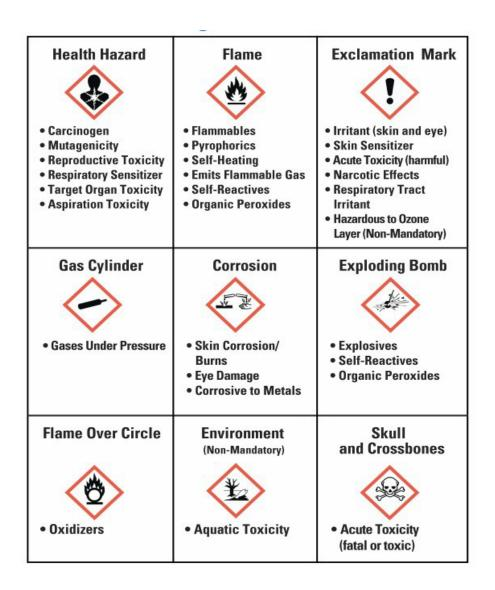
Figure A.VI.1 – Hazard Communication Standard Pictograms
