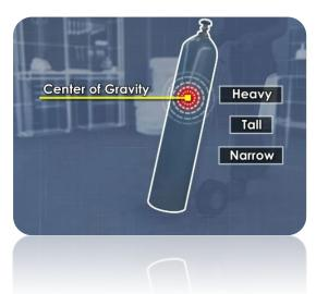
When a typical cylinder is filled to its designed pressure of 2,400 psi, it will contain almost 300  $ft^3$  of atmospheric pressure gas.
