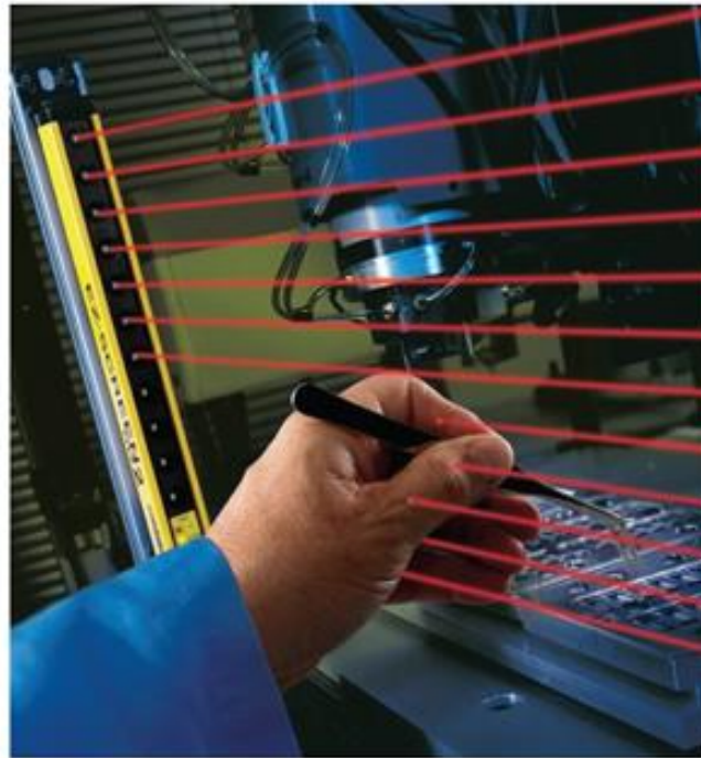
Safety light screens allow safe, unhampered production for a variety of machine-related applications ranging from automated processes to hand-fed machines.
